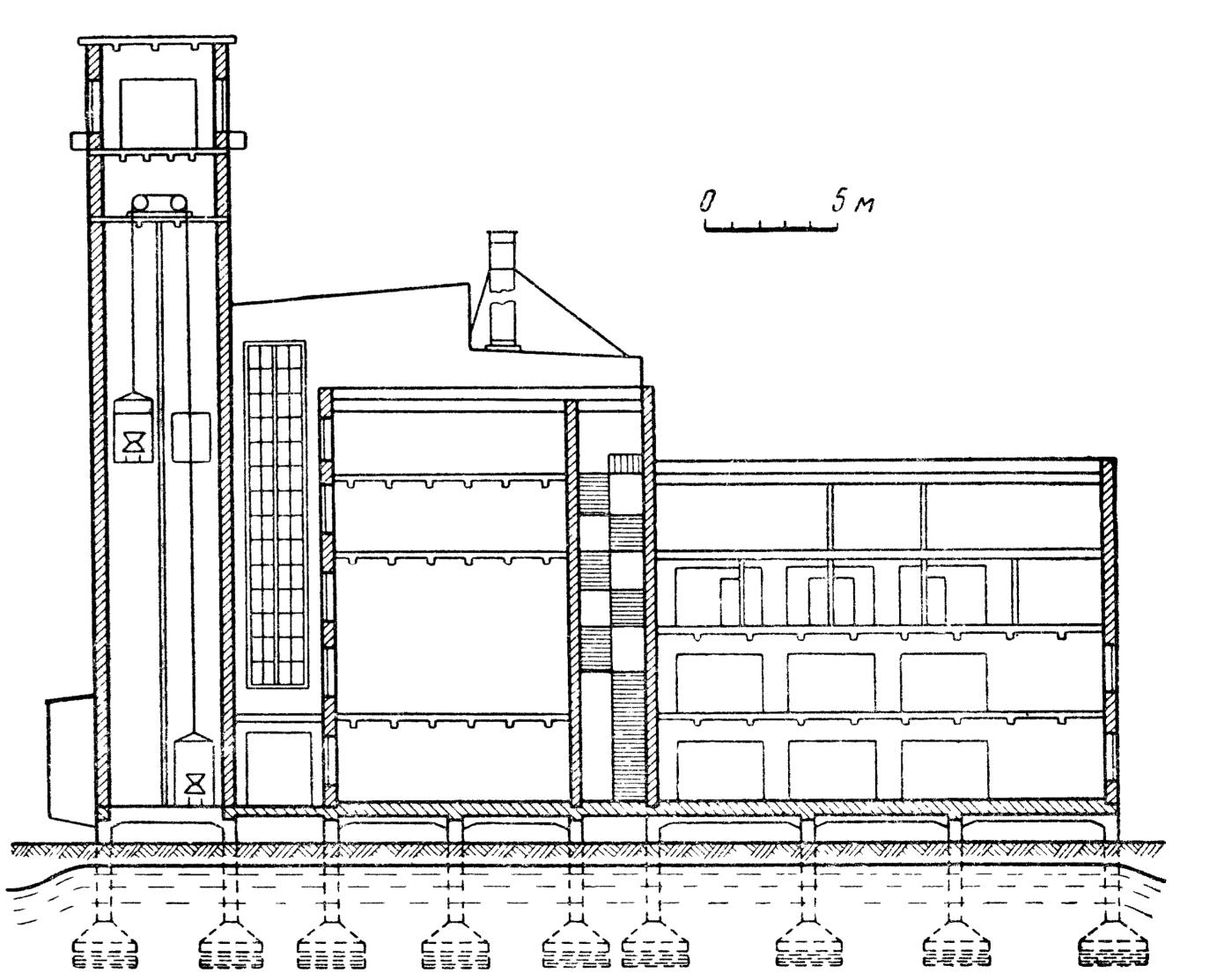
Sectional drawing of the Yakutsk Central Heating Power Plant
